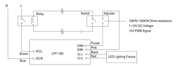
Using a switch and relay can turn  $\ensuremath{\mathsf{ON/OFF}}$  the lighting fixture.
