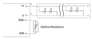
"DO NOT connect "DIM- to -V"
