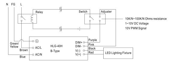
Using a switch and relay can turn  $\ensuremath{\mathsf{ON}}\xspace(\ensuremath{\mathsf{OFF}}\xspace$  the lighting fixture.
