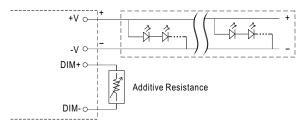
"DO NOT connect "DIM- to -V"
