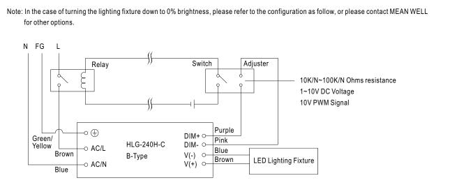
Using a switch and relay can turn ON/OFF the lighting fixture.
