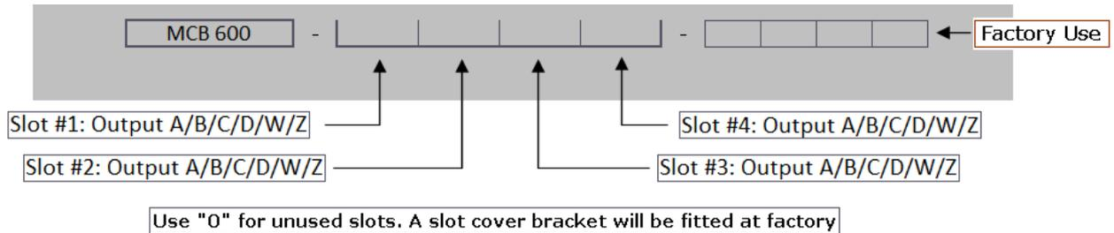
The factory might issue a 4 digit code for a specific configuration which can be used for next and future orders of the same configuration. When ordering an input with no output inserted, simply order "MCB600-XXXX" (Power chassis).
