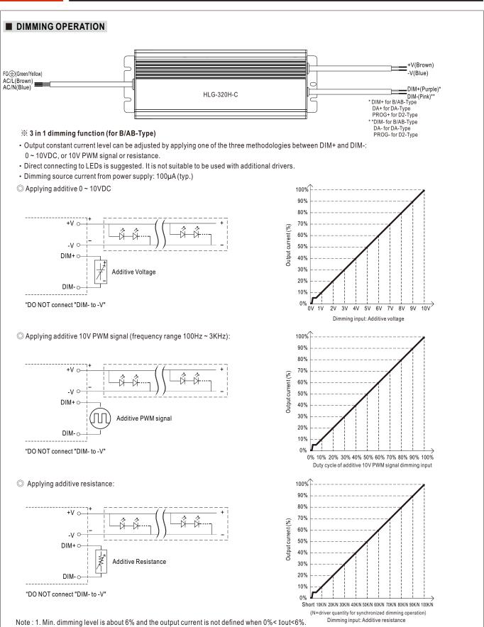
2. The output current could drop down to 0% when dimming input is about 0kΩ or 0Vdc, or 10V PWM signal with 0% duty cycle.
