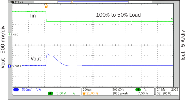
200 \mu s/div rMOR289R5S step load response FIGURE 43
